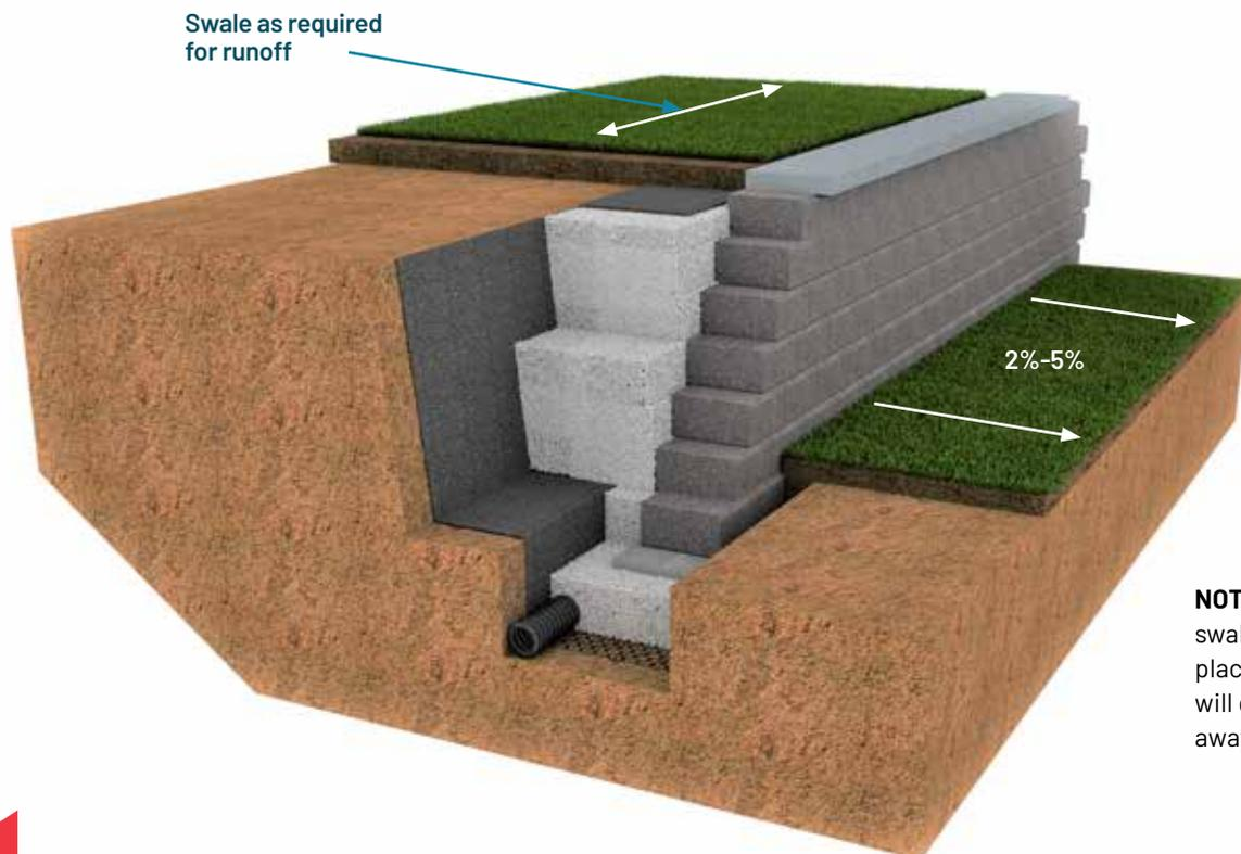
**NOTE:** A carefully graded swale, created before you place the final layer of sod will direct the water flow away from the wall.
