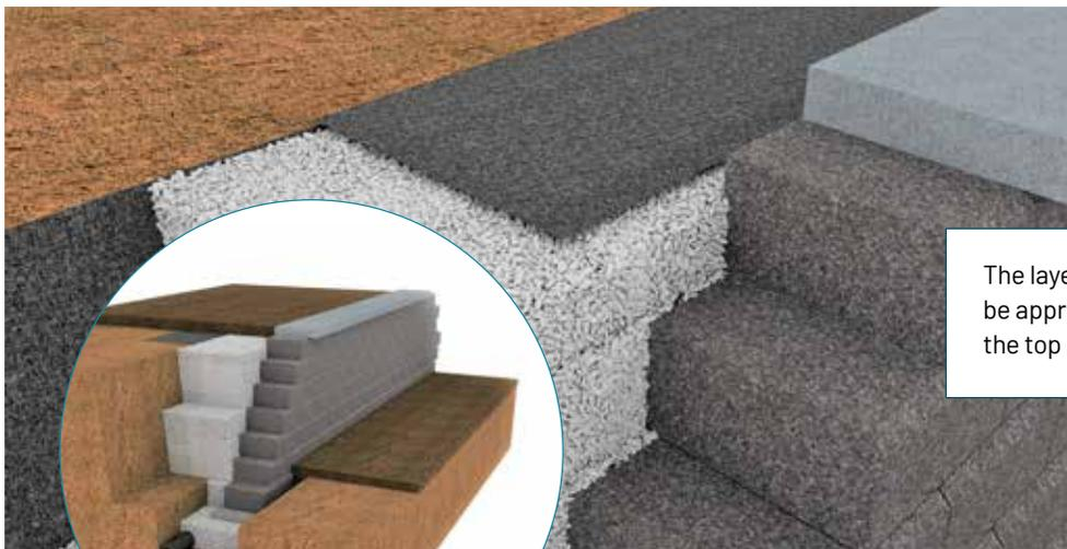
The layer of filter fabric should be approximately 6" (15cm) below the top of the coping.
