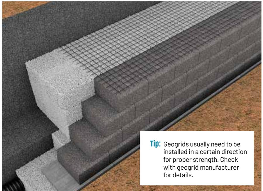
**Tip:** Geogrids usually need to be installed in a certain direction for proper strength. Check with geogrid manufacturer for details.
