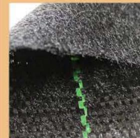
Pro Plus can be used fuzzy side up or down for soil separation, depending on which soil/mulch (top or bottom) needs the stabilization.
