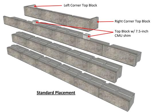
When the standard placement (4-foot face, 2-foot return) is used, it will be necessary for block stability to add a concrete shim beneath the portion of the corner top block that bears over the top block below. This shim is usually made or cut, if necessary, from a standard concrete masonry block (CMU). Gluing this shim in place will resist movement during the backfilling process.
