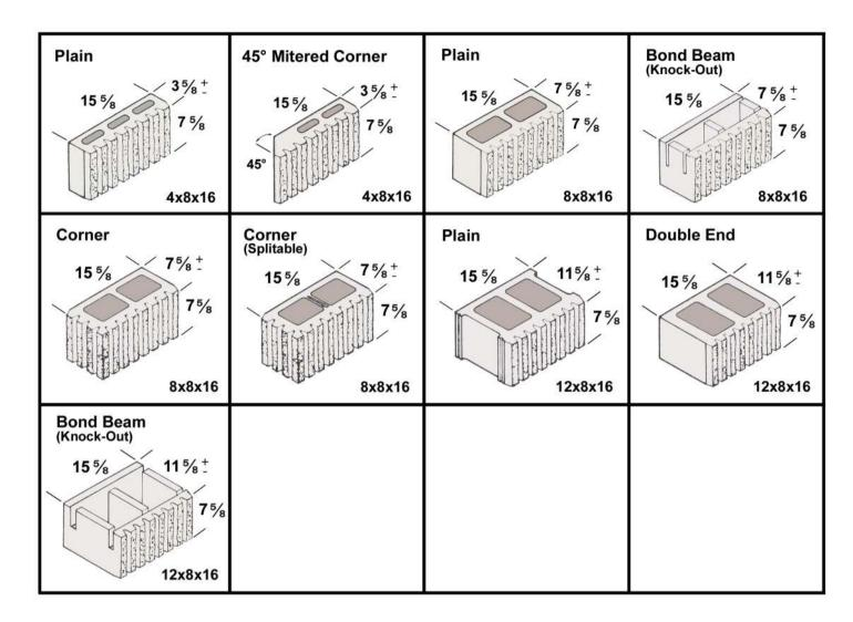
The Corduroy Unit is an eight-fluted exposed aggregate face unit with 7/8" deep grooves, which can be employed in an unbroken wall surface to provide style and interest. The recessed vertical grooves and textured face provide additional visual drama with changing light.
